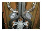
9) Using the included 3/8" bolts, nuts and washers, reconnect the factory side pipes to the new Flowmaster Scavenger assembly. To achieve a more pronounced sound from the side pipes, you may also choose to replace the factory small hole spacer place with the new plates provided with the larger 3/4" holes. Tighten enough to hold but still allow for possible adjustment later.
