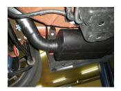
12) Place a 3" clamp onto the inlet pipes of the mufflers. Slide the hanger mounts removed in step 6 onto the new mufflers. Place the mufflers up into position and onto the over-axle pipes, and connect the rear hanger mounts to support. Secure the double hanger mounts back into position on the frame using the factory bolts.
