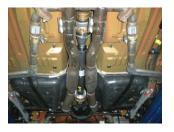
4) Use a 15mm socket to loosen the nuts on the clamped connections at the rear of the factory H-pipe and remove the intermediate pipes. Slip the pipes off and remove from the vehicle.
