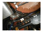
1) Remove the two 15mm bolts that secure the upper panhard bar/brace to the body on the left side, just forward of the muffler. Pull the bar down to gain clearance for muffler removal.
