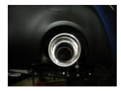
8) Place the **ST339** stainless tips onto both of the exit pipes and adjust to the desired position. Tighten the clamps on the tips enough to hold, but still allow for adjustment.
