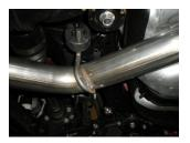
4) Place a provided clamp onto the front of mid-pipe assembly **#16815S** and slide onto the back of the inlet pipe **#16814S**. Rotate the assembly up into its approximate position and connect the hangers on the pipe to their rubber mounts on the vehicle. Tighten the clamp enough to hold, but still allow for adjustment.
