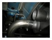
5) Place a provided clamp onto the inlet of muffler #852583-Z and place onto the back of mid-pipe #16815S. Rotate the muffler so that it is level and support the muffler with a stand. Tighten the clamp on the muffler inlet enough to hold, but still allow for adjustment.
