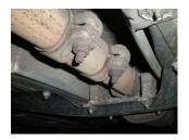
3) At the center of the vehicle, remove the two nuts at the slip-fit connection behind the catalytic converter. Once the connection is loose, separate the two hangers on this section from the rubber mounts on the vehicle and lower the front pipe/resonator from the vehicle.
