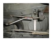
6) Place over-axle pipe **#16835S** into position over the rear axle and slide onto the back of inlet pipe **#16834S**. Connect the hanger on the pipe to the rubber mount on the vehicle and tighten the clamp enough to hold, but still allow for adjustment.
