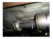
4) Install the muffler inlet pipe **#610TBS** on the back of the factory front pipe. Replace the factory nuts onto the bolts and tighten evenly, tighten enough to hold but still allow for adjustment.
