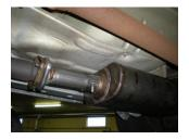
5) Place one of the provided 2½" clamps onto the muffler inlet and then slide the muffler onto the inlet pipe and support with a stand. Tighten the clamp enough to hold but still allow for adjustment. The outlet of the muffler will be toward the inside of the vehicle.
