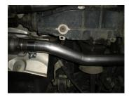
6) Place a provided 2<sup>1</sup>/<sub>4</sub>" clamp onto the right muffler outlet and place the front of pipe **#16901S** into the muffler outlet. Tighten the clamp enough to hold, but still allow for adjustment. Repeat this step on the left side with pipe **#16900S**.
