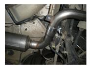
8) Using the 5/16" nuts, bolts and washers provided, attach the cross brace removed from the factory system to the two tabs welded to the mid pipes of the new system.
