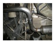
7) Place a provided 2¼" clamp onto the inlet of right side resonator assembly **#15171S** and slide onto the back of pipe **#16901S**. Connect the hanger at the rear of the assembly to the rubber mount on the vehicle and tighten the clamp enough to hold, but still allow for adjustment. Repeat this step on the left side with resonator assembly **#15172S**.
