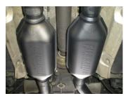
5) Place a provided 2<sup>1</sup>/<sub>4</sub>" clamp onto the inlet of muffler **12412400-Z** and slide onto the right outlet of Scavenger assembly **16896S**. Repeat this step with the other muffler on the left side of the vehicle. Support the mufflers with a stand and tighten the clamps enough to hold, but still allow for adjustment.
