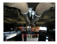
4) Place a provided 2" clamp onto the reduced ends of Scavenger assembly **#16896S**. Place the assembly up into position onto the back of the factory front pipes; connect the hangers at the rear of the assembly to the rubber mounts on the vehicle. Once adjusted, the rubber hangers should be hanging straight up and down. Tighten the clamps at the front of the assembly enough to hold, but still allow for adjustment.
