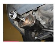
7) Place a provided 2¼" clamp onto the slip-fit of stainless tip **#ST468** and slide it onto the outlet of the right muffler assembly. Adjust to the desired position and tighten the clamp enough to hold, but still allow for adjustment. Repeat this step on the left side of the vehicle.
