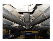
4) Place a provided 2½" clamp onto the expanded end of Y-pipe assembly **#16906S**. Place the pipe up into position onto the back of pipe **#16905S** and connect the hangers on the assembly to the rubber mounts on the vehicle. Once adjusted, the rubber hangers should be hanging straight up and down. Tighten the clamp at the front of the assembly enough to hold, but still allow for adjustment.
