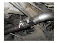
6) Using the 3/8" nuts, bolts and washers provided, attach cross brace **#454HA** to the brackets welded to the right and left muffler assemblies.
