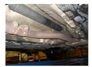
2) Begin by loosening the clamps at the slip connection behind the catalytic converter. Support the rear of the system with stands and starting at the rear, remove the hangers on the system from the rubber mounts on the vehicle. Then, with the help of an assistant, lower the stands and slide the system rearward to remove from the front pipe. Lower the system from the vehicle.
