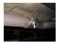
3) Place a provided 2¼" clamp onto the reduced end of inlet pipe #16905S. Place the pipe onto the back of the factory front pipe and rotate to its approximate position in the center channel of the vehicle. Tighten the clamp at the front of the inlet pipe enough to hold, but still allow for adjustment.
