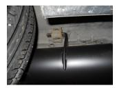
7) Place a provided clamp onto the inlet of muffler **#852460-304.** Connect the hanger on the body of the muffler to the rubber mount on the vehicle and then slide the inlet onto the back of over-axle pipe **#86021S**. Tighten the clamp on the muffler inlet enough to hold, but still allow for adjustment.
