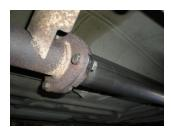
5) Place inlet pipe **#16834S** along with gasket **#GA121** onto the back of the catalytic converter. Using the 3/8" bolts, nuts and washers provided secure the two flanges together and tighten securely. Place a provided 2<sup>1</sup>/<sub>4</sub>" clamp onto the back of this pipe in preparation for the next step.
