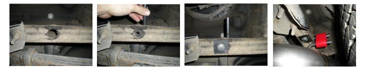
6) On the passenger side of the vehicle, replace the factory rubber hanger mount at the rear of the vehicle with the other supplied HA168 rubber hanger
