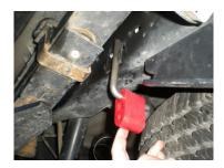
Place a provided 4" clamp onto the expanded end of pipe #46174S, connect the hanger on the pipe to 10) the rubber mount installed in the step above. Then connect the front of the pipe to the rear of pipe #46172S. Confirm that the two pipes are fully slid together and tighten the clamp enough to hold, but still allow for adjustment.
