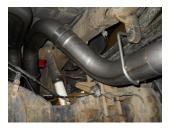
5) Place a clamp onto the expanded end of pipe **#46179S** and slide over the back of pipe #46177S. Connect the hanger on the pipe to the rubber mount on the vehicle and tighten the clamp enough to hold, but still allow for adjustment.
