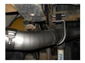
8) Place a clamp onto the expanded end of pipe **#46178S** and slide over the back of pipe **#46176S**. Connect the hanger on the pipe to the rubber mount installed in Step 6 above and tighten the clamp enough to hold, but still allow for adjustment.
