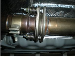
5) Take the provided M10-1.5x60mm bolts and slide on the flat washer. Then, put the bolts thru the flanges and slide on the provided steel spacer sleeves and the springs and nuts removed in step 2 above. Tighten down the fasteners until the nuts bottom out on the steel spacer sleeves.
