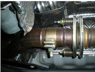
2) Begin by supporting the front and the rear of the system with a stand. Make your way forward from the rear and remove all of the wire hangers on the system from the rubber mounts on the vehicle. Then at the front flange connections, remove the nuts on the spring bolts and set the hardware aside, the springs and nuts will be reused with the Flowmaster system. With the help of an assistant, you can now lower the stands and remove the entire system from the vehicle and set aside.
