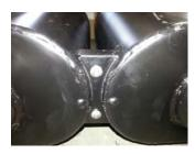
10) Once both mufflers are in place and supported, there are small brackets at the rear that will connect them together. Use the two supplied button head bolts, nuts and washers for this purpose.
