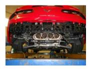
9) Now it's time to start the reassembly process. Position one muffler at a time, up over the axle into the clamps connection. Re-use the original bolts to secure the rear hanger bracket up to the frame.
