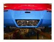
1) Before you begin, please understand that the installation of this system requires significant disassembly. The entire lower rear bumper fascia (Blue portion in photo) must be removed. Because this is a painted body panel, you may want to consider covering it with masking tape for the disassembly/assembly process to prevent any scratches.
