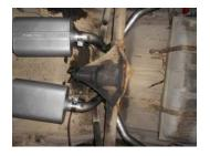
3) Place the **#842546-Z** mufflers into position under the rear seat pan area. Place a clamp onto the muffler outlets. Insert the tailpipes into the muffler outlets and support with stands. Tighten the clamps just enough to hold in position.
