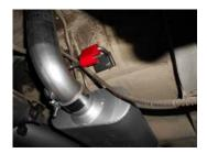
5) Place rubber hangers **#HA168** onto the hanger rods at the front end of the tailpipes. Then connect hanger brackets **#357HA** and **#358HA** to the rubber hangers. See the diagram for proper orientation of brackets. With the mufflers in the proper position, the brackets should fit up against the rear of the seat pan.
