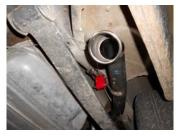
2) Place the right tailpipe **#86191S** over the rear axle so that the rear of the tailpipe exits between the quarter panel and the leaf spring. Repeat this step for the left tailpipe **#86192S**. Connect the hangers on the tailpipes to the rubber mounts installed in the previous step.
