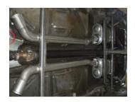
4) Install the front pipe assembly **#86189S** by placing the rear of the front pipe assembly into the inlets of both mufflers and centering it in the drive line cavity. (Be sure to install the clamps first.) Support the front of the assembly with a stand, and position the mufflers and front pipe assembly so that they are level. Once the mufflers and front pipe assembly are in place, check the tailpipe clearance where they go up in front of the rear axle to be sure there is adequate clearance.
