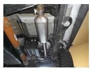
2) Place a provided clamp onto the inlet of muffler **#12518409-Z** and slide over the back of inlet pipe **#710TBS**. Tighten the clamp enough to hold, but still allow for adjustment.
