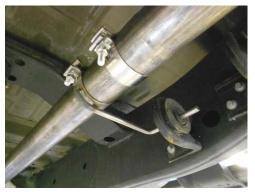
4) Slide the inlet hanger **#490HA** over the back of the inlet pipe and insert the hanger into the factory rubber mount. Do not tighten this clamp yet. If required, place the extension pipe **#26277S** onto the back of the inlet pipe. Then place the inlet of the muffler onto the back of inlet pipe and support with a stand. Level the muffler and tighten the clamp at the inlet enough to hold, but still allow for adjustment.
