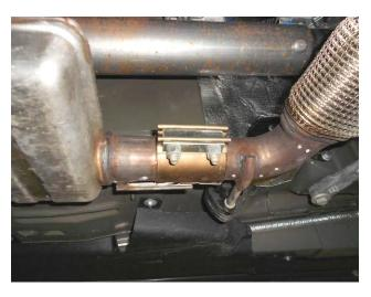
3) Using a 15mm wrench, loosen the two bolts at the clamp connection in the center of the vehicle. Use a small screwdriver to lift the clip and with the help of an assistant, carefully lower the stands at the rear of the vehicle and slide the system toward the rear and off of the front pipe. Lower the system from the vehicle. The clamp should remain on the factory front pipe as it will be re-used with the new Flowmaster system.
