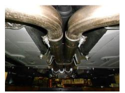
4) Begin the installation by placing a supplied 2-3/4" clamp onto each of the inlets of the Scavenger pipe **#26522S**. Then place the Scavenger pipe onto the back of the stock head pipes (the offset outlet pipe should be oriented to the right side). Level and center the assembly in the drive line tunnel and support with a stand. Tighten the two clamps enough to hold, but still allow for adjustment.
