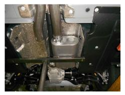
5) Place a supplied 3" clamp onto the inlet neck of both mufflers. Slide the mufflers onto the back of the Scavenger pipe assembly and support with stands. Level the mufflers and tighten the clamps enough to hold, but still allow for adjustment.
