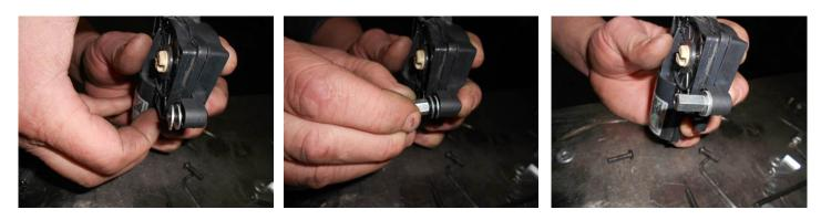
2) The actuator with the spacers and spring attached.
