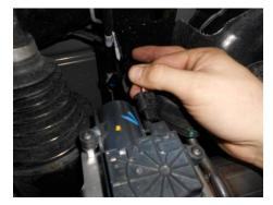
7) Reconnect the two electrical plugs removed in step 2 of the removal instructions back onto the tailpipe actuators now installed on the new Flowmaster tailpipes.
