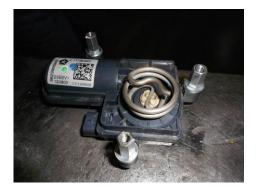
3) Place the actuator assembly against the bracket on the new Flowmaster tailpipe as shown in the first photo below, the center arm of the spring will be between the tabs on the bracket. Rotate the assembly so that the actuator motor is upright and until the spacers line up with the holes in the bracket. Install the included  $\#10-32 \times 3/8$ " Button Head Screws from the back of the bracket and into the spacers and shown in the third photo below. Tighten securely.
