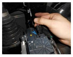
7) Reconnect the two electrical plugs removed in step 2 of the removal instructions back onto the tailpipe actuators now installed on the new Flowmaster tailpipes.
