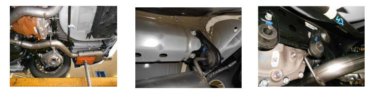
2) Place the right muffler assembly **#843045-407** up into position and slide the inlet completely onto the factory pipe. Support the assembly with a stand and remount the rear hanger mount to the frame and tighten securely. Remount the front hanger to the cross member and tighten securely. Leave the clamp on the inlet loose for now. Repeat this step with muffler assembly **#843045-406** on the left side of the vehicle.
