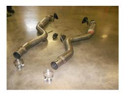
1) Place the new Flowmaster muffler assemblies next to the factory units and swap the front and rear hanger mounts from the stock mufflers to the Flowmaster assemblies. Place a provided 2.25" clamp onto the inlet of each assembly. Tighten the clamp just enough to hold in place.
