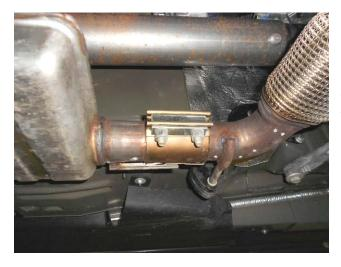
3) Using a 15mm wrench, loosen the two bolts at the clamp connection in the center of the vehicle. Use a small screwdriver to lift the clip and with the help of an assistant, carefully lower the stands at the rear of the vehicle and slide the system toward the rear and off of the front pipe. Lower the system from the vehicle. The clamp should remain on the factory front pipe as it will be re-used with the new Flowmaster system.
