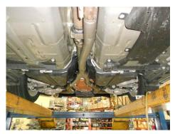
2) Place the Y-pipe assembly **#86320S** up into position behind the factory front pipe and slide into the clamp until it stops. Support the rear of the Y-pipe with a stand and tighten the clamp enough to hold, but still allow for adjustment. The Y-pipe outlet with two bends will be oriented to the drivers' side of the vehicle.
