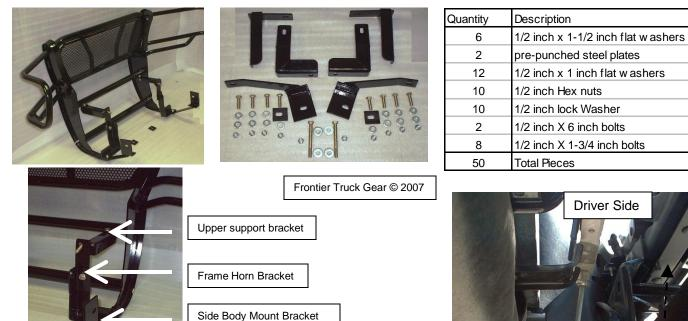
**Step 1:** Pull out plastic pegs that hold rubber flap on the bottom, but <u>do</u> <u>not remove rubber</u>. Remove plastic punched grate from bumper opening on both sides (if installed).
