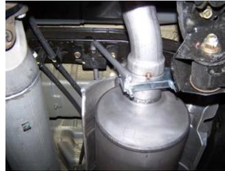
6. Next, install rear muffler hanger #F onto outlet of muffler. Insert hanger into rubber grommet. Do not tighten.
