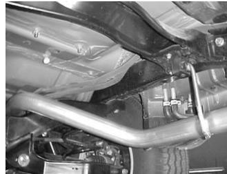
7. Install overaxle tailpipe #C into muffler 1.5"-2". Secure to the muffler using clamp #F. Do not tighten.
