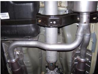
3. Install Y-pipe #A onto your existing stock flanges. Insert hanger into rubber grommet. Use your factory hardware to secure. Do not tighten.
