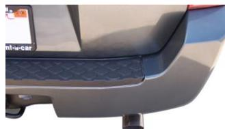
8. Install stainless steel tip. Clamp down. When you have everything in place, firmly tighten all bolts and clamps down securely. Start from the front of the system and work your way back. Use stainless steel cleaner and a Scotch Brite pad weekly to prevent tip from discoloration. Inspect all fasteners after 25-50 miles of operation and re-tighten as necessary.
