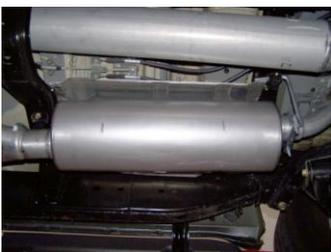
4. Install muffler #B onto headpipe #A 1.5"-2" with the louvers facing towards the converter. Use a jack stand to support the muffler. Use clamp #E to secure the muffler to the headpipe. Do not tighten. Muffler inlet is looking into the louvers. Outlet of muffler will be at the one o'clock position.
