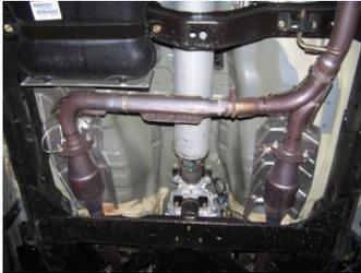
2. To remove the stock exhaust, unbolt the 2-bolt flanges located in front of your factory muffler. Next, unbolt your stock tailpipe behind your muffler. Do not discard your factory hardware, you will reuse it. (May need to remove spare tire for easier removal of tailpipe.)
