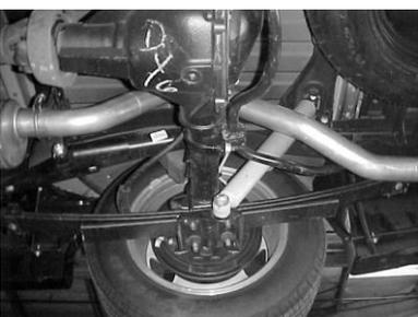
INSTALL OVERAXLE TAILPIPE #C INTO MUFFLER AT LEAST 1 1/2" TO 2". SHORTER END GOES IN TO MUFFLER. SPARE TIRE MIGHT HAVE TO BE LOOSENED AND PUSHED OVER TOWARDS THE DRIVERS SIDE FOR BETTER CLEARANCE. ATTACH TO CLAMP #H.
