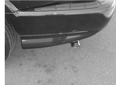
INSTALL STAINLESS TIP. USE ANY STAINLESS CLEANER TO CLEAN TIP. YOU CAN NOW TIGHTEN ALL NUTS, BOLTS, FLANGE AND CLAMPS STARTING FROM THE FRONT AND WORKING YOUR WAY TO THE BACK
