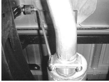
BOLT ON THE HEADPIPE #A USING FACTORY GASKET #J AND ATTACH WITH BOLT KIT #I. THE END OF THE HEADPIPE SHOULD BE AT APPROX. 7 O'CLOCK POSITION. DO NOT TIGHTEN. USE CLAMP #G TO SECURE MUFFLER TO HEADPIPE. DO NOT TIGHTEN. ATTACH MUFFLER HANGER #F INTO RUBBER GROMMET. AND INSERT WELDED HANGER INTO RUBBER GROMMET.
