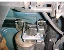
Install rear muffler hanger #D onto outlet of muffler. Do not tighten.
