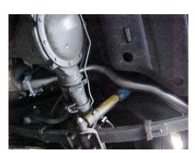
Install the overaxle tailpipe #B. Attach to muffler with hanger #D, Insert welded hanger into factory rubber grommet. For easier installation raise vehicle with jack by the frame. Then install tailpipe as seen in picture.
