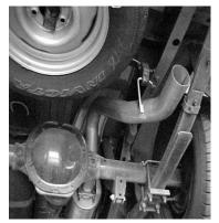
INSTALL OVER AXLE PIPE #B INTO THE OUTLET OF THE MUFFLER 1-1/2" TO 2". INSERT REAR WELDED HANGER INTO THE FACTORY RUBBER GROMMET ATTACH HANGER #G AND CLAMP #E AT THE OUTLET OF THE MUFFLER. DO NOT TIGHTEN.
