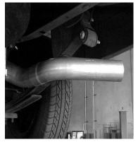
INSTALL EXIT PIPE #C ONTO THE OVER AXLE PIPE USING CLAMP #E. DO NOT TIGHTEN. NOW ROTATE PIPE'S UNTIL YOU HAVE A MINIMUM OF A 1" CLEARANCE ON ALL PIPE'S. THEN TIGHTEN ALL CLAMPS AND HANGERS.
