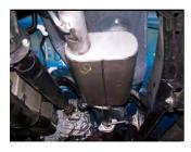
**3.** Install muffler #B onto head pipe 1½"-2" with the louvers facing towards the converter. Use a jack stand to support the muffler. Use clamp #E to secure the muffler to the headpipe. DO NOT TIGHTEN.
