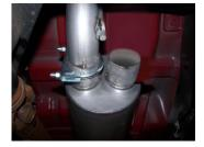
5. Install driver side over axle tailpipe #C into muffler 1.5-2". Use clamp #G to secure tailpipe to muffler. DO NOT TIGHTEN.
