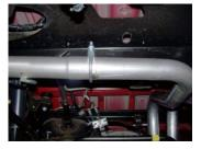
6. Install driver side exit pipe #D onto over axle tailpipe. Use clamp #G to secure. DO NOT TIGHTEN. Insert welded hanger into rubber grommet.
