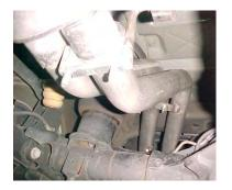
Install the passenger side over axle tailpipe # D into the muffler 1-1/2" to 2". Insert welded hanger into rubber grommet. Use clamp # J to secure pipe to muffler, do not tighten.
