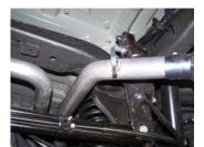
5. Slide the passenger side over axle tailpipe #C into the muffler 1.5-2". Use clamp #G to secure tailpipe to muffler. Do not tighten. Insert welded hanger into rubber grommet.
