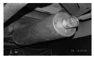
SLIDE MUFFLER ONTO HEADPIPE 1-1/2" TO 2" USING CLAMP #F TO SECURE MUFFLER TO HEADPIPE. USE A JACKSTAND TO SUPPORT MUFFLER. DO NOT TIGHTEN. MUFFLER INLET IS LOOKING INTO THE LOUVERS.
