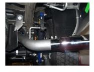
6. Install stainless steel tip. Clamp down. When you have everything in place, firmly tighten all bolts and clamps down securely. Use stainless steel cleaner and a Scotch Brite pad weekly to prevent tip from discoloration. Inspect all fasteners after 25-50 miles of operation and re-tighten as necessary
