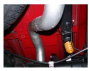
5. Install the overaxle tailpipe #C onto the outlet of the muffler 1.5"-2" using clamp #E to secure pipe to muffler. Insert welded hanger into rubber grommet.
