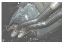
2. To remove the stock exhaust measure 4" from the factory flange on both head pipes towards the rear of the vehicle and cut. Disengage the welded hangers from the rubber grommets using WD-40 to aid in this process. Do not damage or remove the rubber grommets as you will re-use them to mount the new system.
