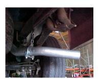
Next, install the exit pipes # E. Use clamps # I to secure to the tailpipes, and attach hangers' # J.
