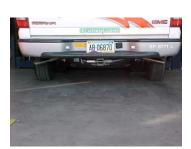
Install stainless steel tips. Clamp down. When you have everything in place, firmly tighten all bolts and clamps down securely. To clean stainless steel tips, use stainless steel cleaner and a Scotch Brite pad. Use zip ties to tie away brake lines.
