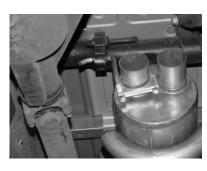
INSTALL MUFFLER #B ONTO HEADPIPE, AT LEAST 1 ½" TO 2". USE CLAMP #F TO SECURE MUFFLER TO HEADPIPE. DO NOT TIGHTEN. USE A JACK STAND TO SUPPORT THE MUFFLER. OUTLETS SHOULD BE AT THE TOP. INSTALL REAR MUFFLER HANGER #I ONTO DRIVERSIDE MUFFLER OUTLET AND INSERT WELDED HANGER INTO GROMMET. DO NOT TIGHTEN.
