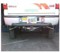
INSTALL EXIT PIPES #E ONTO TAILPIPES AND ATTACH TO HANGER #H AND CLAMP #G TO SECURE EXIT PIPES TO TAILPIPES. THESE METAL HANGERS NEED TO BE ROTATED IN ORDER TO ADJUST FOR CLAMPING. CUT TO YOUR PREFERED LENGTH. NOW INSTALL YOUR STAINLESS STEEL TIPS TO YOUR DESIRED LOOK. NOW YOU CAN TIGHTEN ALL CLAMPS, NUTS, AND BOLTS. STARTING FROM THE FRONT WORKING BACK, USE ZIP TIES TO TIE AWAY BRAKE LINES.
