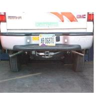
INSTALL PASSENGER SIDE TAILPIPE (#C) INTO MUFFLER AT LEAST 1  $\frac{1}{2}$ " TO 2". USE CLAMP #G TO SECURE PIPE TO MUFFLER. DO NOT TIGHTEN. THE TAILPIPES WILL BOTH LEAN TOWARDS THE DRIVER SIDE LOOKING FROM THE REAR OF THE VEHICLE.
