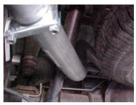
INSTALL DRIVER SIDE TAILPIPE (#D) INTO MUFFLER AT LEAST 1 ½" TO 2". THIS PIPE WILL ROUTE OVER THE AXLE, BETWEEN THE SHOCK AND SPARE TIRE. ATTACH CLAMP #g TO SECURE TAILPIPE TO MUFFLER. DO NOT TIGHTEN. LOOKING FROM INSERT WELDED HANDER INTO RUBBER GROMMET.
