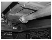
BOLT HEADPIPE #A TO THE STOCK FLANGE RE-USING FACTORY NUTS. DO NOT TIGHTEN. SLIDE WELDED HANGER INTO RUBBER GROMMET
