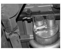
INSTALL THE MUFFLER (#B) ONTO HEADPIPE AT LEAST 1½" TO 2". USE CLAMP (#F) TO SECURE MUFFLER TO HEADPIPE. DO NOT TIGHTEN. USE A JACK STAND TO SUPPORT THE MUFFLER. OUTLETS SHOULD BE AT THE TOP. INSTALL HANGER #I ONTO DRIVERSIDE MUFFLER OUTLET AND INSERT WELDED HANGER INTO GROMMET. DO NOT TIGHTEN.
