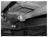
BOLT HEADPIPE (#A) TO THE STOCK FLANGE RE-USING FACTORY NUTS. DO NOT TIGHTEN AND CONNECT WITH CLAMP (#F). SLIDE WELDED HANGER INTO RUBBER GROMMET. INSTALL THE HEAD PIPE EXTENSION (#J).
