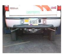
INSTALL EXIT PIPES #E ONTO TAILPIPES AND ATTACH TO HANGER #H AND CLAMP #G TO SECURE EXIT PIPES TO TAILPIPES. THESE METAL HANGERS NEED TO BE ROTATED IN ORDER TO ADJUST FOR CLAMPING. CUT TO YOUR PREFERED LENGTH; NOW INSTALL YOUR STAINLESS STEEL TIPS TO YOUR DESIRED LOOK. NOW YOU CAN TIGHTEN ALL CLAMPS, NUTS, AND BOLTS. STARTING FROM THE FRONT AND WORKING BACK. USE ZIP TIES TO TIE AWAY BRAKE LINES.
