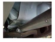
Install head pipe (#A) onto you're existing stock flange use your factory hardware. Use a jack stand to support the converter.
