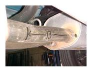
Lay out the exhaust on the floor so it looks like the drawing and compare parts with manual. To remove the stock exhaust cut 13" just in front of the muffler. Leave all rubber grommets in place. Use WD-40 to aid in removal of exhaust and hangers. Use hacksaw to cut tailpipe off.
