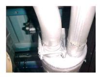
Next, install rear muffler hanger (#**H**) onto driver's side muffler outlet and insert hanger into rubber grommet. Do not tighten.
