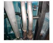
Install driverside headpipe (#B). Then install headpipe (#A) and insert welded hanger into rubber grommet. Secure both pipes with clamp (#G). Do not tighten.
