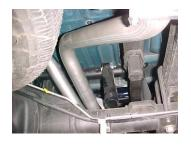
Install the passenger side over axle tailpipe (**#D**) into muffler 1 ½" to 2". Secure with clamp (**#I**). Do not tighten.
