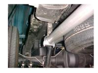
Install tailpipe hangers (#J) onto end of tailpipes using clamp (#I). There will be about a 2" hole above the end of both tailpipes on the frame to bolt the hangers. Do not tighten.
