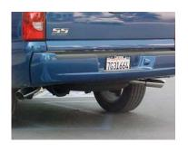
INSTALL EXIT PIPES # F ONTO TAILPIPES. CUT 10" OFF EACH TAILPIPE, USE CLAMPS # I TO SECURE EXIT PIPES TO TAILPIPES. THESE CLAMPS ALSO ATTACH TO METAL HANGERS # J. THESE METAL HANGERS NEED TO BE ROTATED IN ORDER TO ADJUST FOR CLAMPING. ROTATE EXIT PIPES TO POINT OUT TO THE SIDE. NOW YOU CAN TIGHTEN ALL CLAMPS, NUTS, AND BOLTS. STARTING FROM THE FRONT WORKING BACK. INSTALL STAINLESS TIPS. USE ZIP TIES FOR BRAKE AND FUEL LINES..
