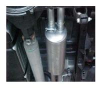
INSTALL MUFFLER #C ONTO HEADPIPES 1 ½" TO 2". USE CLAMP #G TO SECURE MUFFLER TO HEADPIPES. DO NOT TIGHTEN. OUTLETS SHOULD BE AT THE TOP. SUPPORT MUFFLER WITH A JACK STAND.
