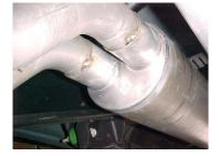
Install muffler# C onto head pipes 1-1/2" to 2" with the louvers facing towards the converter. Outlets will be on top. Use a jack stand to support the muffler. Use clamps #G to the secure the muffler to the head pipes. Do not tighten
