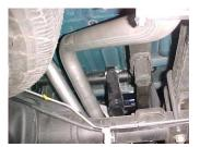
Install passenger side overaxle tailpipe #D into muffler 1  $\frac{1}{2}$ " to 2". Secure to muffler with clamp #H. Do not tighten.
