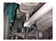
Install tailpipe hangers #I onto end of tailpipes using clamp #H. There will be about a 2" hole above the end of both tailpipes on the frame to bolt the hangers. Do not tighten.
