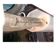
Lay out the exhaust on the floor so it looks like the drawing and compare parts with manual. **To** remove the stock exhaust cut 13" just in front of the
