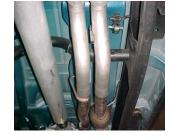
Install driverside headpipe #B onto factory pipe. Then install headpipe #A onto factory pipe and insert welded hanger into rubber grommet. Secure both pipes with clamp #G. Do not tighten.
