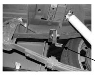
INSTALL HANGER # F ON THE PASSENGER TAILPIPE AND HANGER # G ON DRIVERSIDE TAILPIPE. MEASURE 19" FROM REAR OF FRAME AND BOLT INTO THE EXISTING ROUND HOLES (ABOUT 7/8") LOCATED ON THE FRAME ON BOTH SIDES OF THE VEHICLE.
