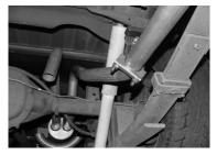
INSTALL PASSENGER SIDE TAILPIPE # C INTO THE MUFFLER 1-1/2" TO 2". ATTACH IT TO THE MUFFLER USING CLAMP # I USE CLAMP # I TO HOLD TAILPIPE TO HANGER # F. DO NOT TIGHTEN
