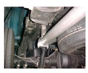
**9.** Install tail pipe hangers #H onto end of tail pipes using clamp #G. There will be about a 2" hole above the end of both tail pipes on the frame to bolt the hangers. Do not tighten.
