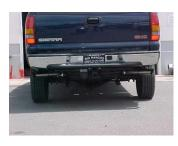
**10.** Install exit pipes #F. Use clamps #G to secure exit pipes to tail pipes. Clamps #G also attach to metal hangers #H. Install stainless steel tips. When you have everything in place, firmly tighten all bolts and clamps down securely. Use stainless steel cleaner and a Scotch Brite pad weekly to prevent tip from discoloration. Inspect all fasteners after 25-50 miles of operation and re-tighten as necessary.
