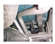
**8.** Install passenger side over axle tail pipe #C into muffler 11/2-2". Secure with clamp #G. Do not tighten.
