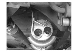
Install muffler # B with the inlet towards the converter onto the head pipes at least 1-1/2" to 2" using clamps #F. Use a jackstand to support. The inlet of the muffler should be at about 6'oclock.Do not tighten.
