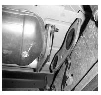
Unbolt stock flange behind the rear of the converter. You will reuse the stock bolts. Remove stock hangers leaving rubber grommets in place. Use WD-40 on hangers for easier removal. Cut & remove the stock tailpipe.
