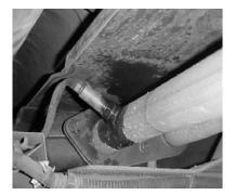
Remove O2 sensor from stock head pipe and remove stock flange gasket. You will reuse the stock bolts.
