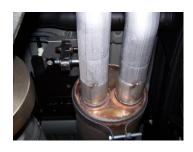
**5.** Slide passenger side tail pipe #C into muffler 1½ - 2". Use clamp #F to secure tail pipe to muffler. Do not tighten.
