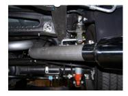
6. Install passenger side tailpipe #C into muffler 1.5-2". Use clamp #H to secure pipes together. Do not tighten. Insert welded hanger into rubber grommet.
