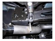
8. Install exit pipe #E onto the tailpipe 1.5-2" and secure with clamp #H. Do not tighten. Rotate pipe to best suit your vehicle. Insert welded hanger into rubber grommet. Adjust pipes to fit your vehicle with tips on so you make sure there is proper clearance.
