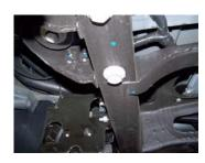
7. Install rear tailpipe hanger #1. Remove hitch bolt as seen in picture. Insert rubber grommet on hanger.
