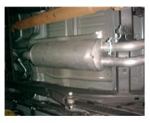
INSTALL MUFFLER # B ONTO HEAD PIPE 1-1/2"-2" WITH THE LOUVERS FACING TOWARDS THE CONVERTER. USE A JACK STAND TO SUPPORT THE MUFFLER. USE CLAMP # G TO SECURE THE MUFFLER TO THE HEADPIPE. DO NOT TIGHTEN.
